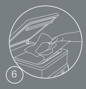
Removing the packaging After vacuuming and sealing, the chamber lid opens automatically.
