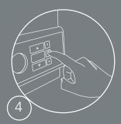
Selecting the program Select one of the three defined programs, or enter a sealing time and vacuuming time in accordance with requirements.
